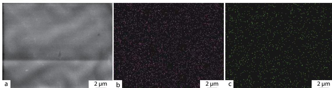
Fig. 5 (a) SEM image of the elastomer with an Al-to-COOH ratio of 0.01:1 and an Eu-to-IDA ratio of 0.2:1 (Eu-to-Al molar ratio of 0.35:1). The (b) Al and (c) Eu element-distributions analyzed by an EDX from the region in (a).
